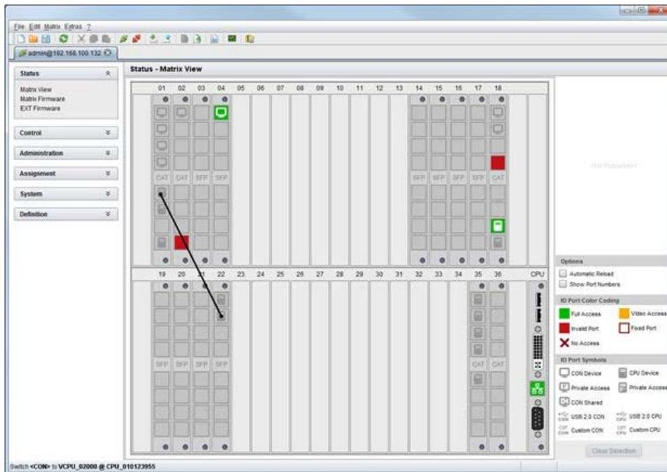
Figure 68. Extended KVM Switching through Java Tool - Method 2 (from Matrix View Option)
