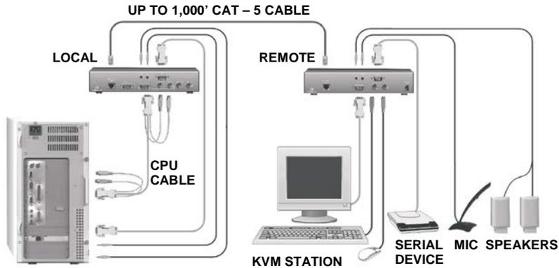
Figure 8. Serial/Audio model cabling
