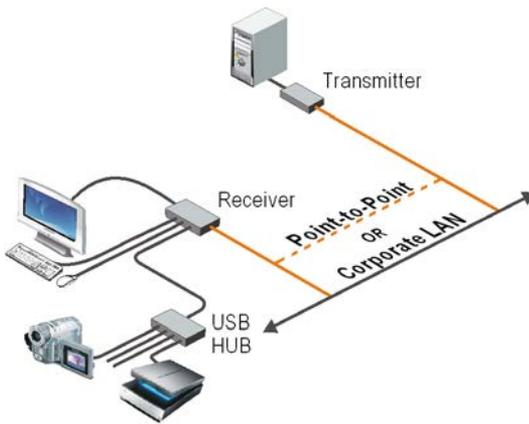
**Figure 2. Typical Installation**
