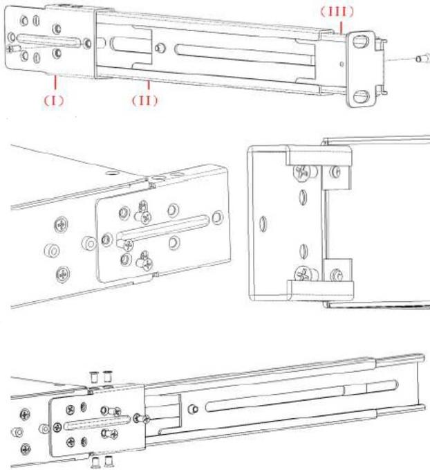
5. When the rack depth is greater than 680mm (26.77") with Rackview 15" and 17", and greater than 745mm (29.33") with the Rackview 19".
