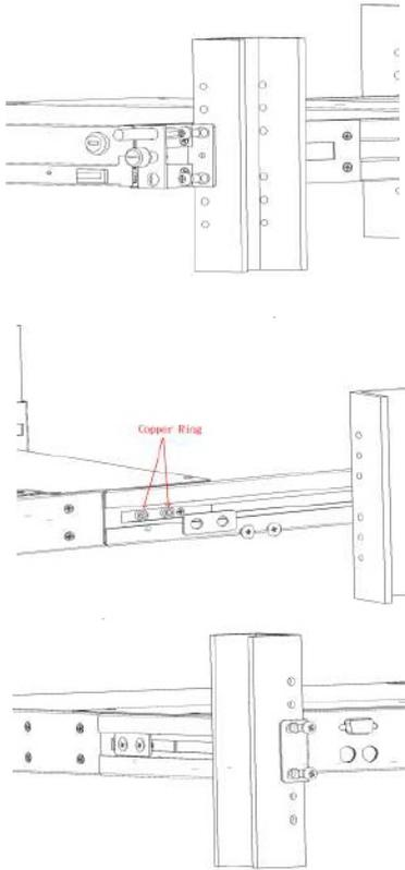
4. For a rack depth above 535mm (21.06") with Rackview 15" and 17", and for a rack depth above 595mm (23.42") with the Rackview 19".
