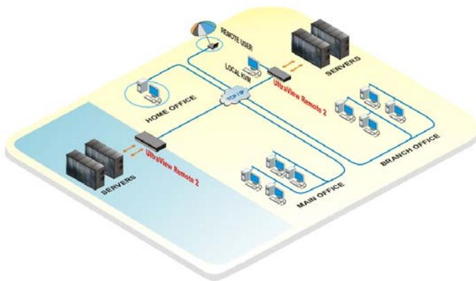
**UltraView Remote 2 Model** The UltraView™ Remote 2 is available in an 8, and 16 port version. UltraView Remote 2 can be chained together with our UltraView Pro or ServView Pro to support up to 256 computers.
