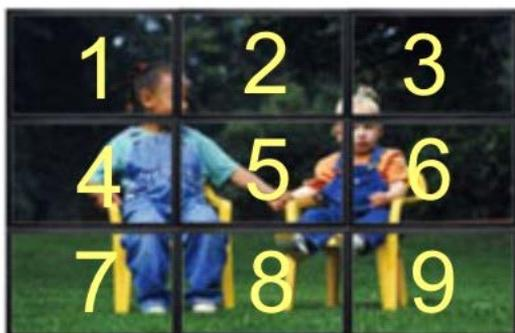
Figure 21. 3 x 3 array for VWL-B133FD
