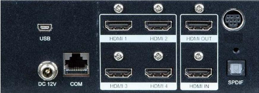
Figure 3. Rear Panel Connectors
