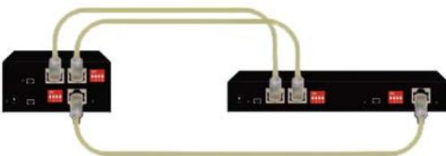
CATx cabling is connected as shown to the left. Up to 150 ft. max.
