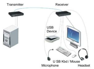
Figure 2. Connectivity Diagram
