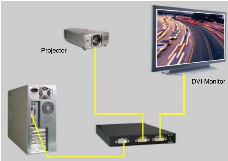
**Figure 2. Basic Installation**
